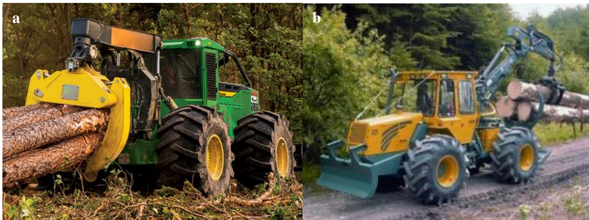
Figure 90. Skidder with a) a grapple and b) a clam bunk (photos: John Deere Forestry and HSM).
