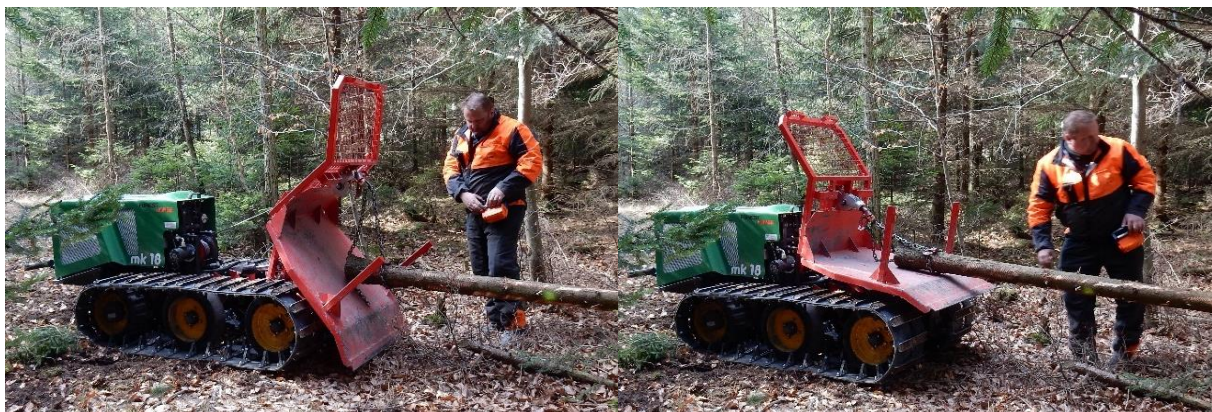
Figure 85. A small skidding tracked machine MK-18 and its use (photos: Engineering Blatná s.r.o.).
