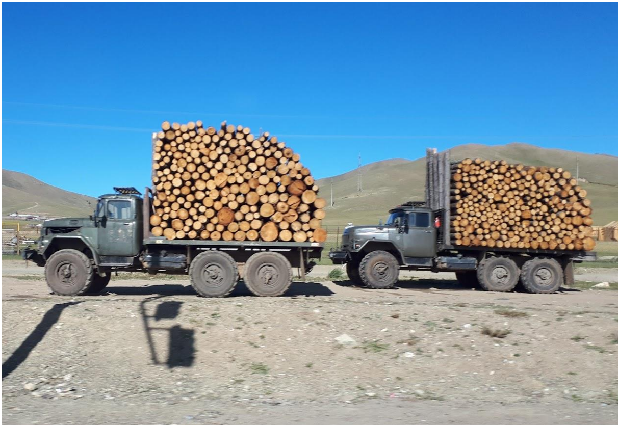
Figure 108. The ZIL-131 is a general purpose 3.5 tonne 6×6 army truck designed in the Soviet Union by ZIL. The basic model is a general cargo truck and local people in Mongolia often use the truck to transport wood (author: Ján Parobek).
