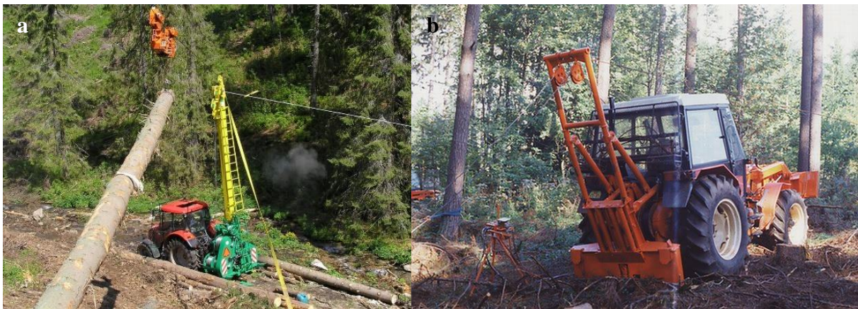
Figure 92. Examples of cable systems: a) cable transport installations and b) adapter (short tractor) cable system (photos: University Enterprise MFK MENDELÚ).
