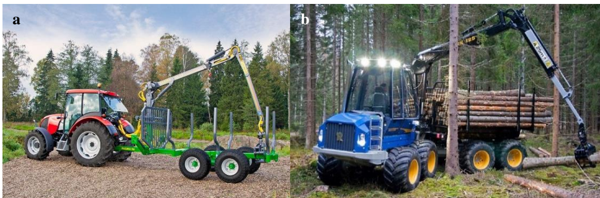
Figure 91. Timber forwarding machines: a) tractor and trailer unit and b) forwarder (photos: AGAMA a.s. and Rottne).
